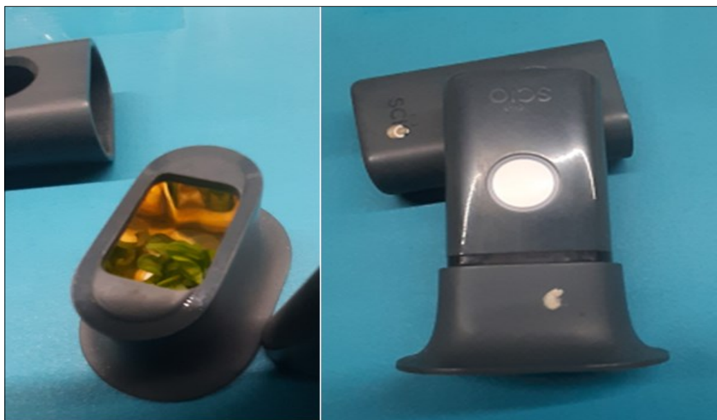
Figure 3. Scanning the leaves, after measuring the pH, with the SCiO™ device
